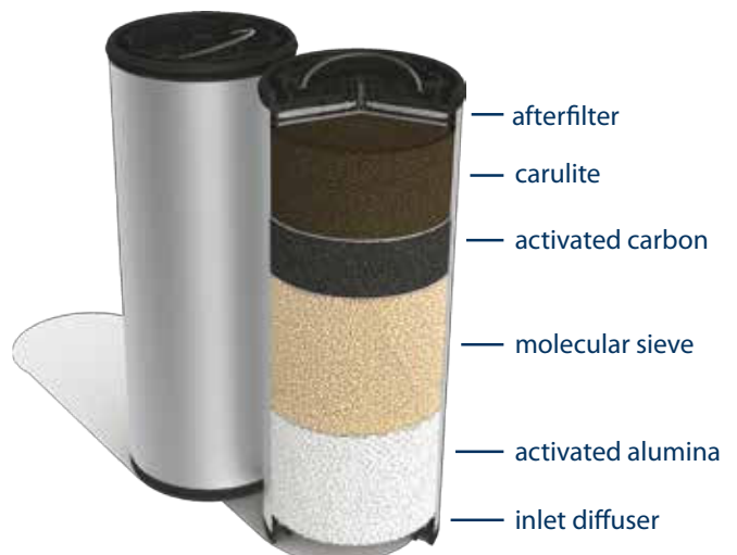
4-layer mixed bed cartridge
